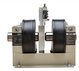
The MK50 electromagnet is coupled with the MPSK-50 bipolar power supply. This power supply is capable of providing 12 Amps of current at 36 volts (400 Watts). It is continuously controllable over both the current and voltage range windows, and is controlled by the MMR Technologies Hall Measurement software and the Hall Measurement Controller.
